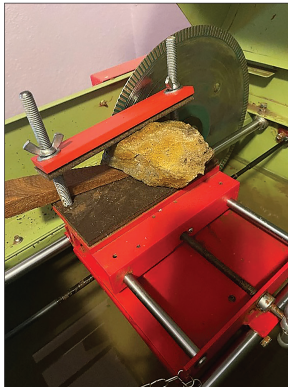
Slab Saw used to slice large rocks.
