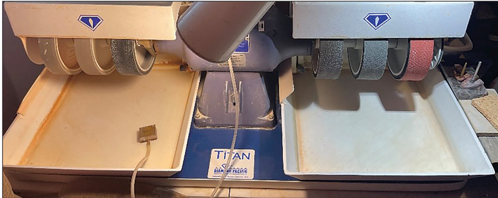
Cabbing Machine used for shaping and polishing cabochons.
